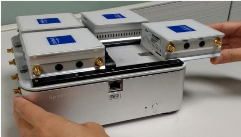
**Figure 12.** Landslide E10 – Module Carrier Plate
