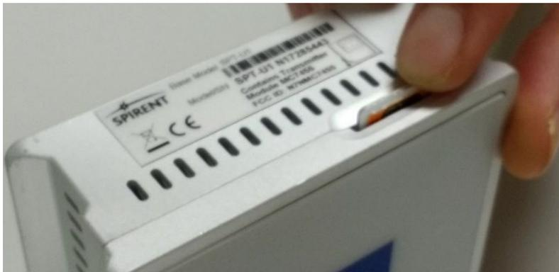
**Figure 8.** Landslide E10 – SIM Card Insertion and Removal
