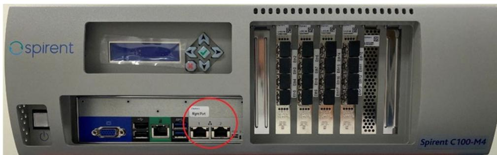
**Figure 2.** Landslide (C100-M4) Front Panel - Management Port
