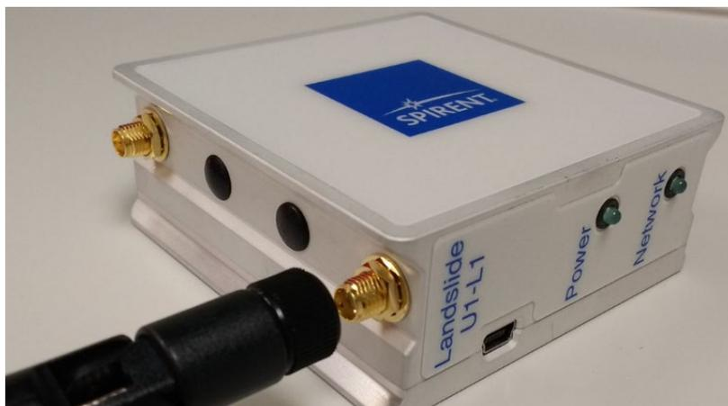
**Figure 17.** Connecting the Antenna to the U1 OTA Module
