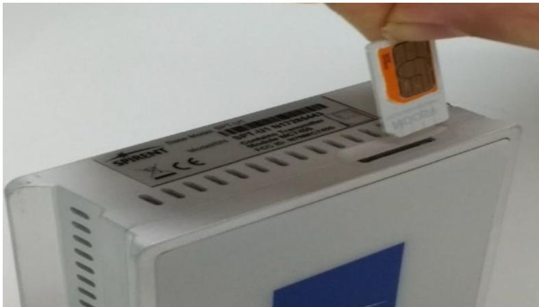
**Figure 7.** Landslide E10 – SIM Card Insertion and Removal
